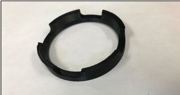
Figure 6: Joint Light Tactical Vehicle (JLTV) Slotted Bushing.
